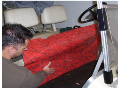
WARNING: Film will not stick to flaking paint or highly oxidized paint. In extreme cases buffing may be needed
